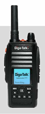
The DTP-9750 is the workhorse of the Diga-Talk+ spectrum of offerings. Leveraging the power of LTE, you get private and group calling, on-device recording and playback, GPS tracking, and over-the-air programming. The four quick keys on the front make accessing your favorite group or individual as simple as pushing a button. The 9750 makes for a reliable communications companion that will work for you across the street or across the nation.
